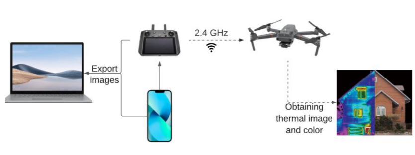
Figure 6. Obtaining photos using Drone.
