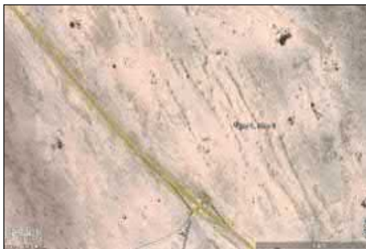
Day 1-Figure 09. Dammam formation ridges oriented North-South along the Dukhan highway over the Dukhan anticline.
